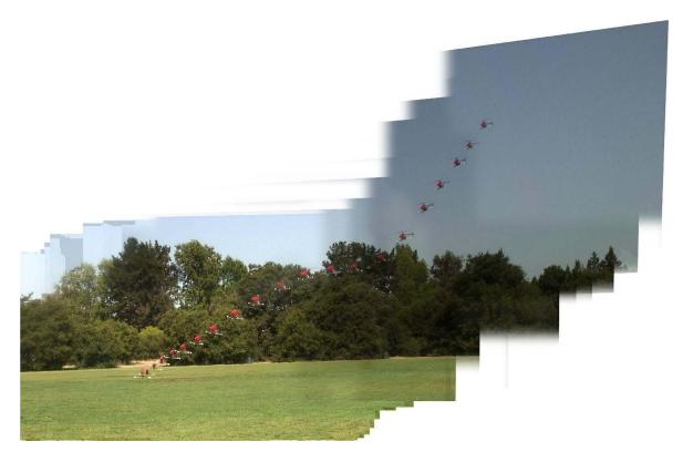
Suppose you are using machine learning to teach a helicopter to fly complex maneuvers. Here is a time-lapse photo of a computer-controller helicopter executing a landing with the engine turned off.
